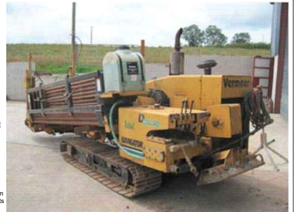
Directional Drilling Rig
